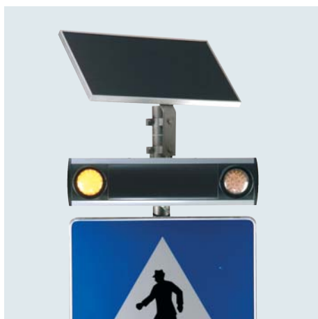
Signflash 630 - Solar Flashing LED unit, width 630 mm, integrated control unit and battery
